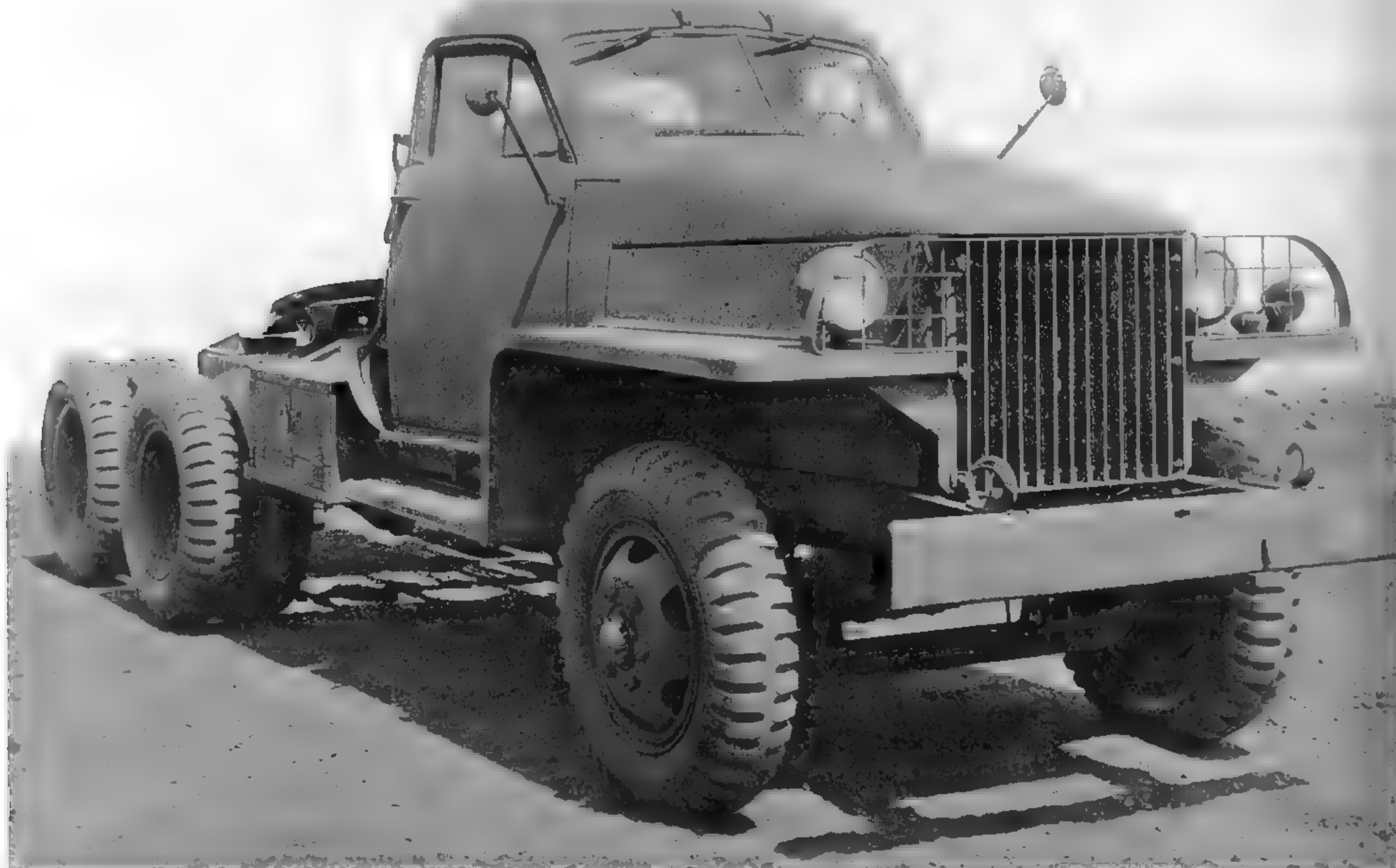
All the G-630 series trucks were not six-wheel drive, as can be seen in this view of a Studebaker model US6 6x4 short-wheelbase tractor. Cargo trucks were also built with non-powered front axles. (U.S. Army photo)
